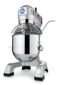
Powerful planetary mixer Robust stainless steel bowl of 20.0L 3 speeds: 105 - 180 - 408 RPM Strong machine with high speed Strong transmission with metal gears Bowl lift with lever and safety switch Stainless steel protective guard over the bowl Safety switch in the guard Separate start and stop buttons Cast-iron casing with scratch-resistant coating Very easy to clean Available in 'Grey Deluxe'
